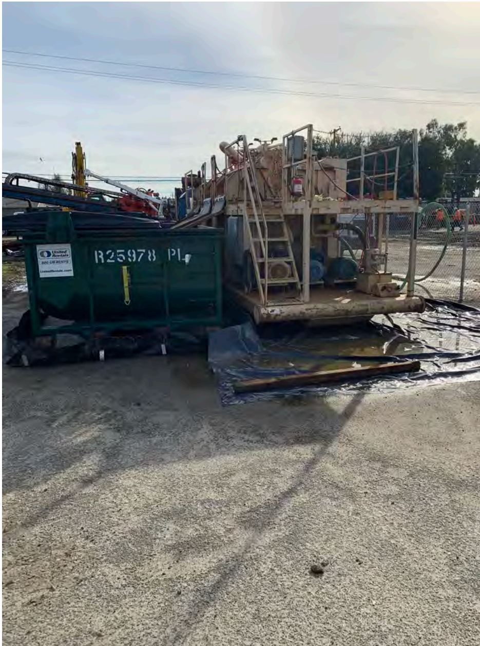
Photograph 2: View of mud system (MCT800), looking south.
